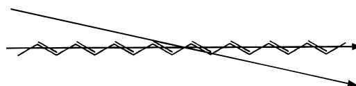
Figure 1. A linear conjugated polyene structure with an arrow illustrating the transition dipole orientation with an off-axis angle of magnitude determined by experiment and a sense indicated by theory. The long axis of the polyene is also shown.
